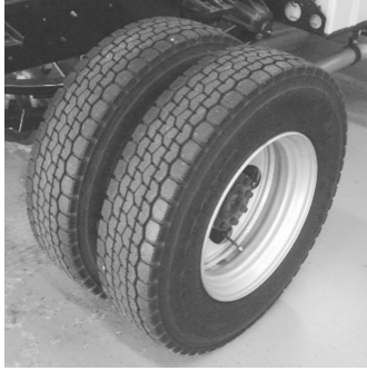
Fig.2 Double-tire construction (rear axle)
