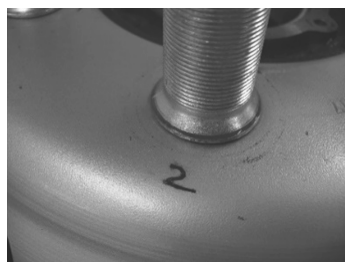
Fig.14 Line contact mark generated on the contact surface of an inner nut
