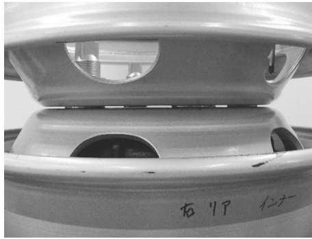
Fig.13 Generated gap between an inner wheel and an outer wheel
