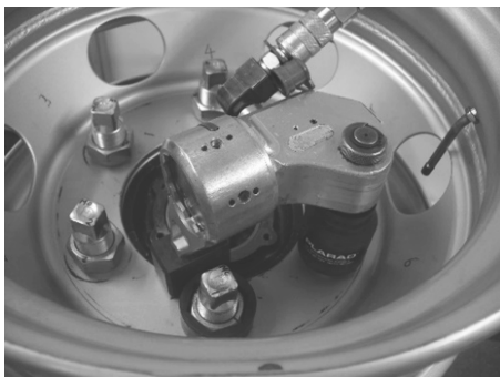
Fig.4 Inner nuts and outer nuts tightened by oil pressure wrench
